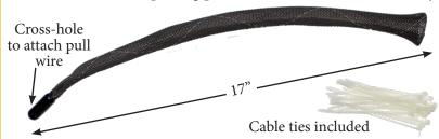
secure a cable tie near the connector, and pull your cable. The pull tension will grab and secure the wire while the double-walled construction safely protects your connectors. Expands to fit up to 1-3/4" dia. of wire, contracts down to 3/4" dia.
