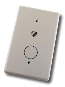
The GRI Door Alert Annunciator is designed to signal customer entry into a business establishment. A closed loop magnet reed switch activates the Door Alert. It can be set by the installer for a two, four or six second sounding time. Offered in a recessed version (easily mounted in a single gang box) or as a surface mount version. Both units can be powered by an external 12 volt DC power source or 9 volt battery.
