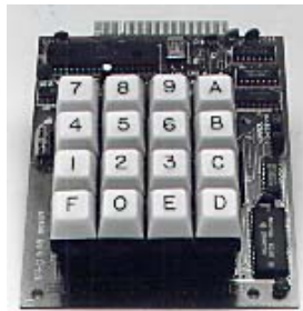
9016 with KB illuminated switches, Alignment Blocks, and Lexan keycaps
