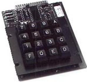
9016 with KBM switches, mounting frame and ABS keycaps
